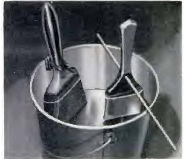
Above, two methods of suspending brushes in solvent. Brushes should not be allowed to rest on bottom of can, as resulting curled bristles cannot be straightened
